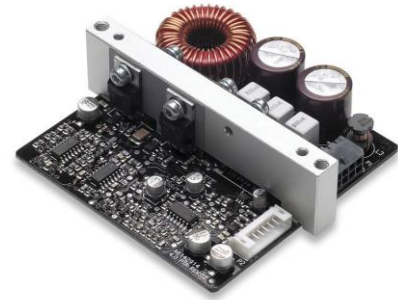
Figure 1: ICEpower500A Size: 9 x 9 x 2.7cm
